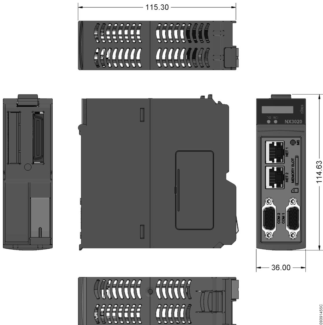
Figure 23: 36 mm NX3020 CPU module
