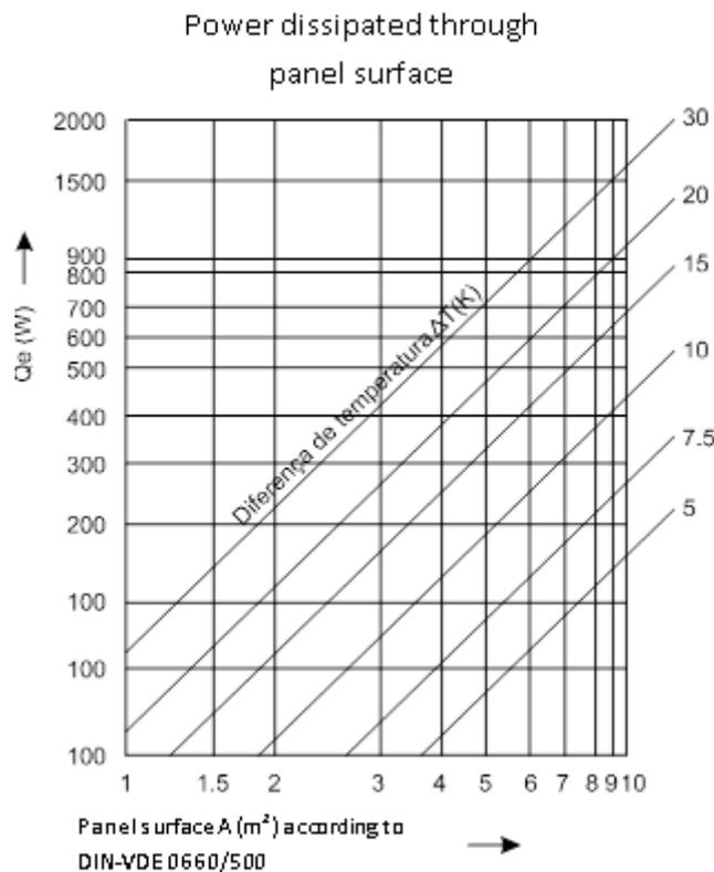
Figure 32: Dissipated Power x Surface x Temperature difference
