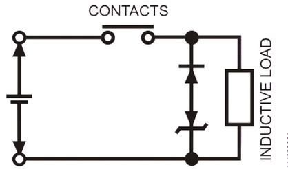
Figure 36: Zener diode circuit
