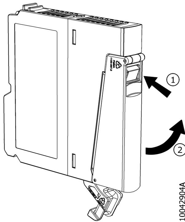
Figure 59: Movement to Remove the I/O Connector Block Nexto Modules
