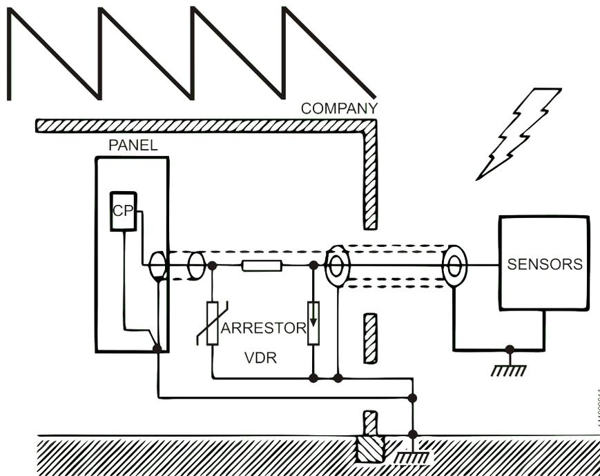
Figure 42: Protection against lightning
