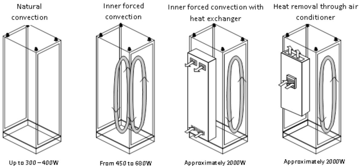
Figure 33: Example of Heat Flow – Closed Installation
