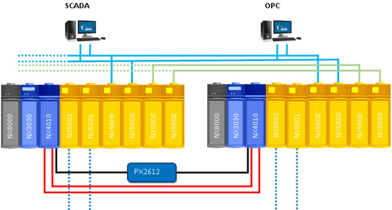
Figure 13: NX3030 - CPU Redundancy
