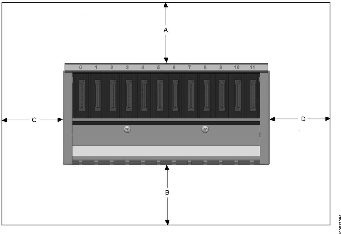
Figure 31: Free space around the PLC
