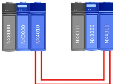
Figure 14: Minimum Configuration of a Redundant PLC - NX3030
