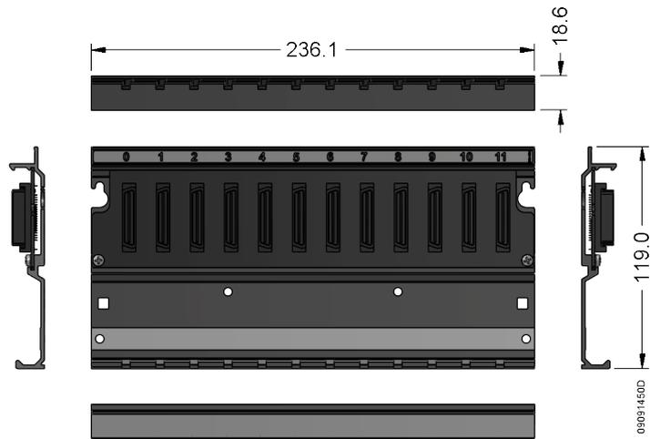
Figure 27: 12-Slot Backplane Rack
