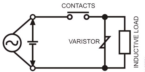
Figure 37: Varistor circuit
