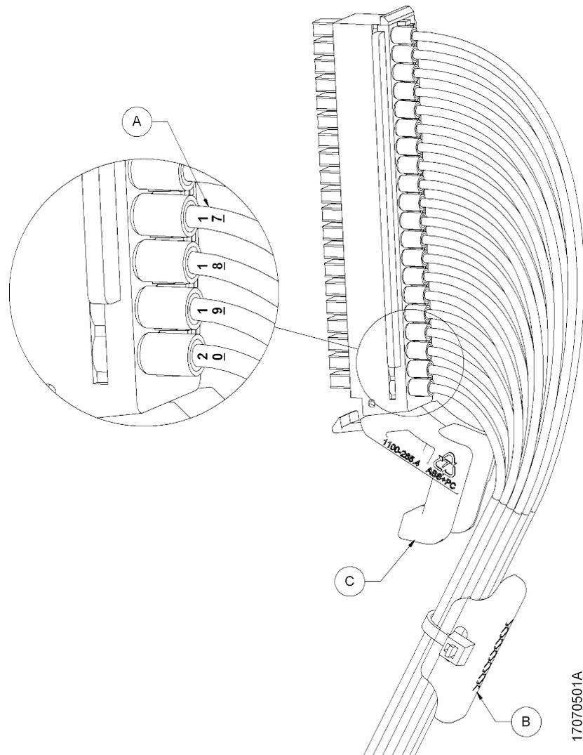
Figure 76: Nexto Jet Cabling ID and Fixation
