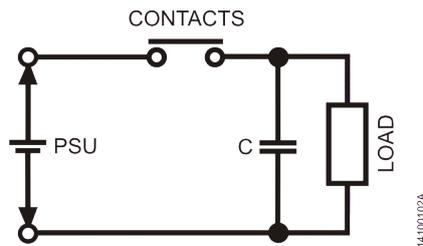
Figure 41: Circuit with capacitor in parallel with the load
