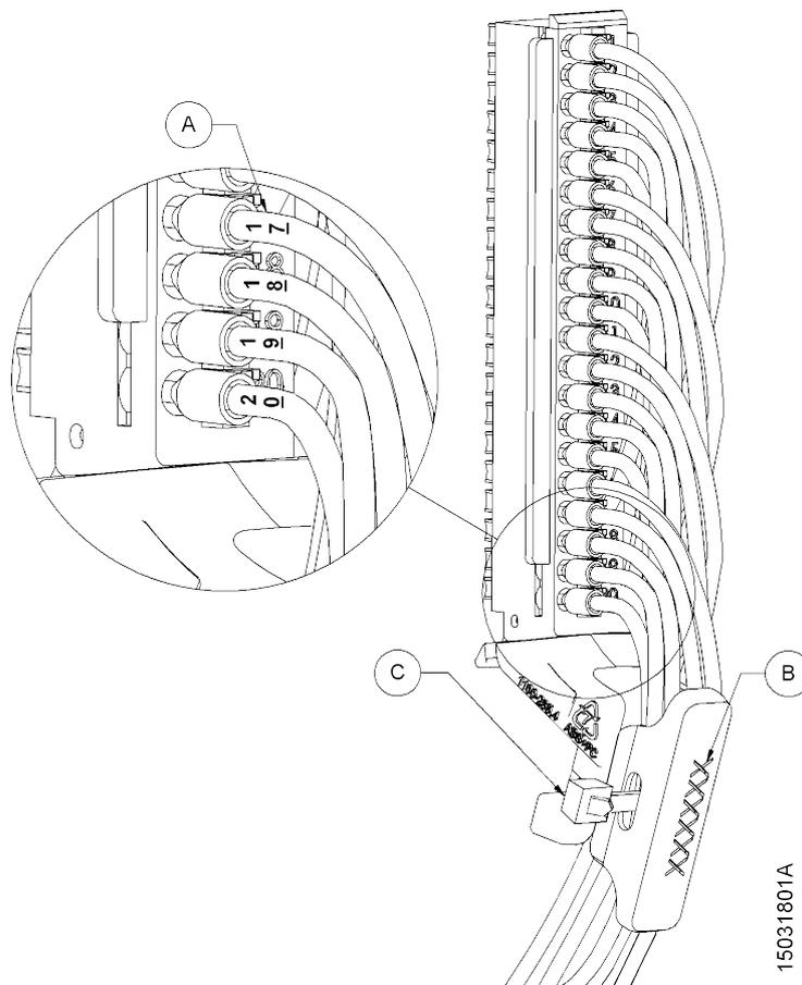
Figure 75: Nexto Cabling ID and Fixation
