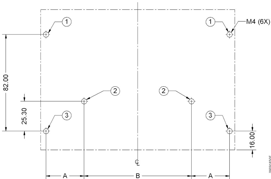
Figure 43: Drilling for Rack Fixation
