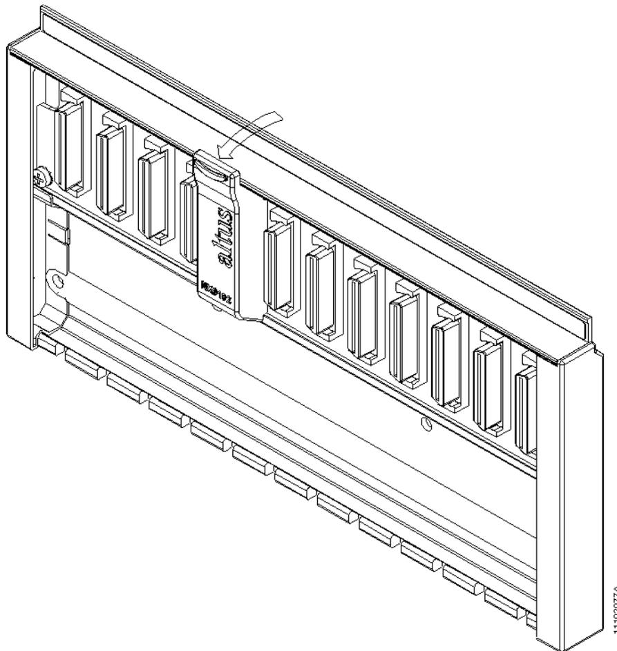
Figure 69: Rack Connector Cover Removal
