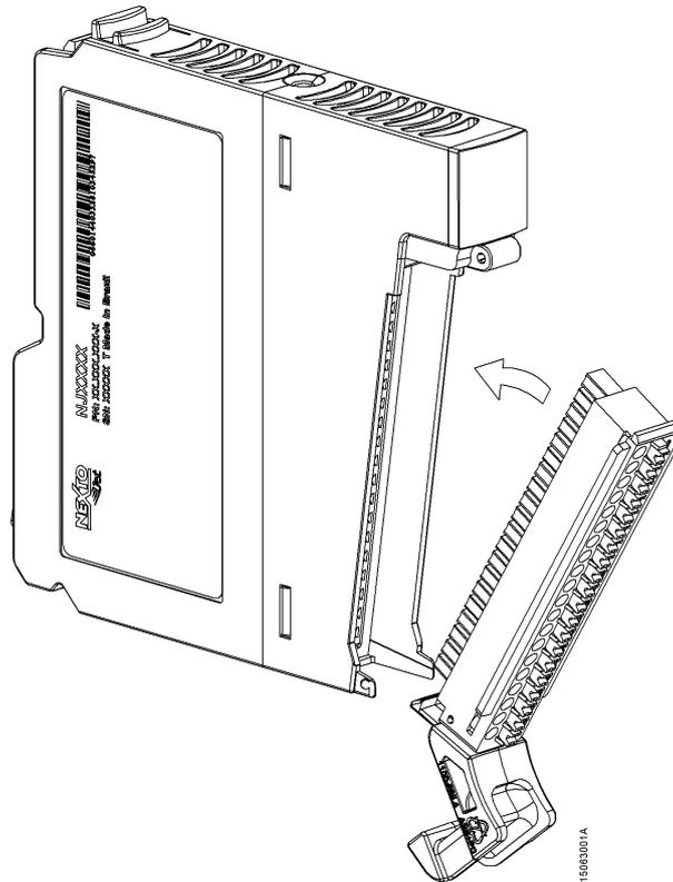
Figure 58: Insertion of Nexto Jet Connector
