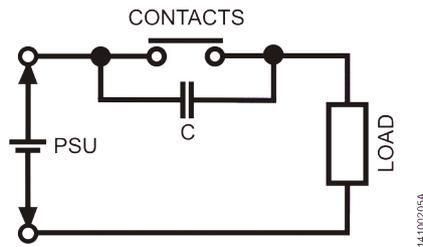
Figure 40: Circuit with capacitor in parallel with contacts
