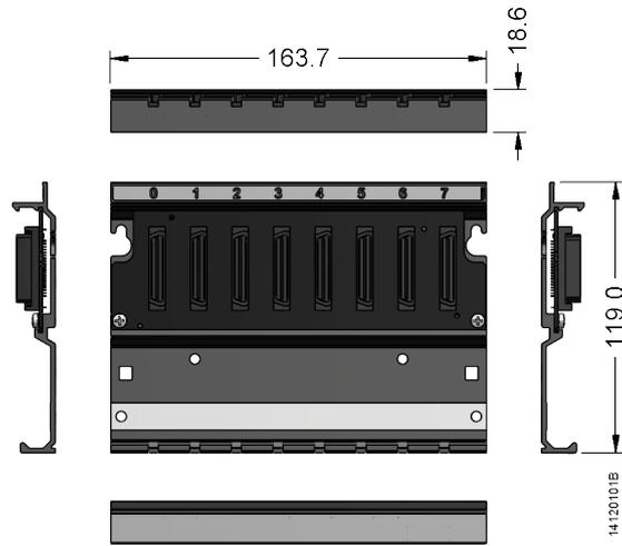
Figure 26: 8-Slot Backplane Rack
