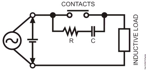
Figure 38: RC circuit parallel with contacts
