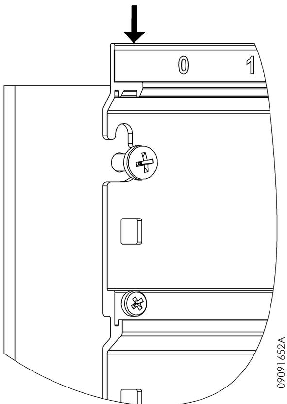
Figure 46: Rack fixation – Keyway fitting
