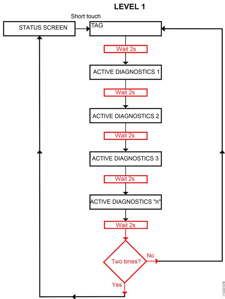
Figure 77: CPU Diagnostics Visualization
