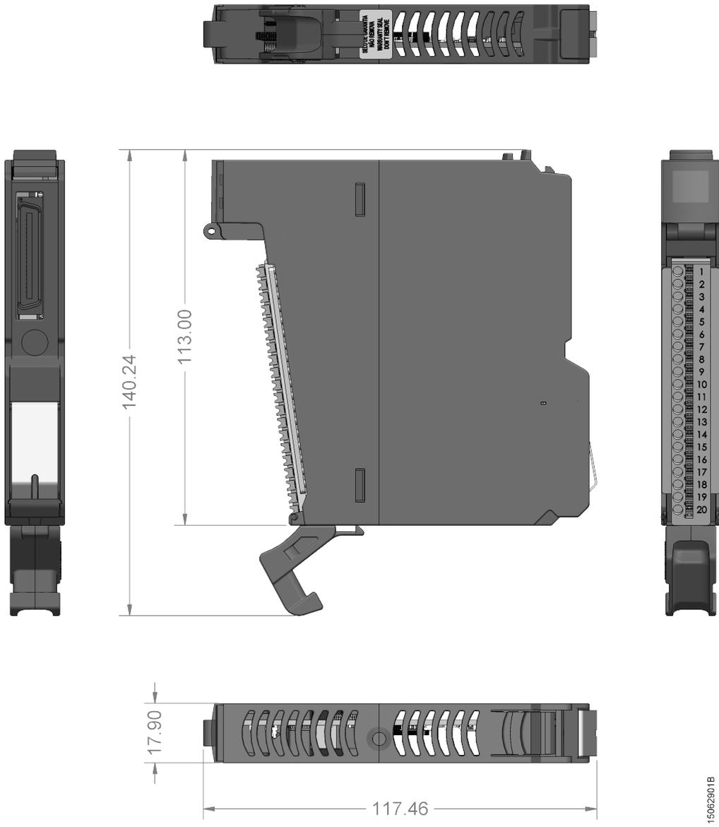
Figure 21: Nexto Jet 18mm I/O Module
