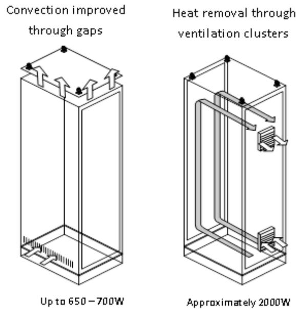
Figure 34: Example of Heat Flow – Open Installation
