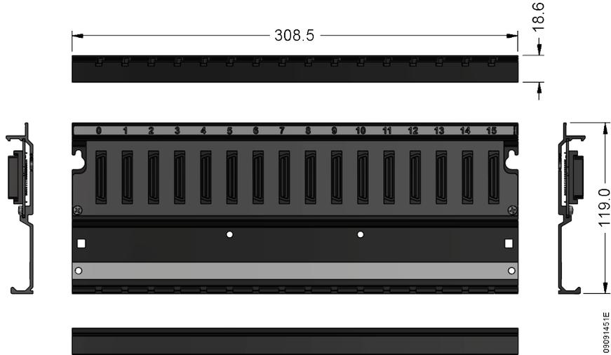
Figure 28: 16-Slot Backplane Rack
