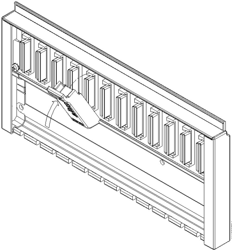
Figure 68: Rack Connector Cover Insertion
