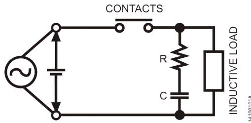
Figure 39: RC circuit parallel with the load
