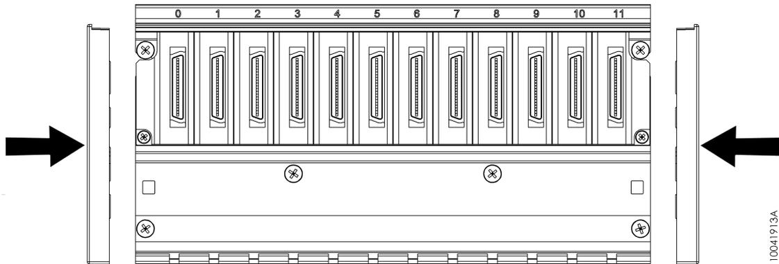
Figure 47: Rack fixation – Side covers
