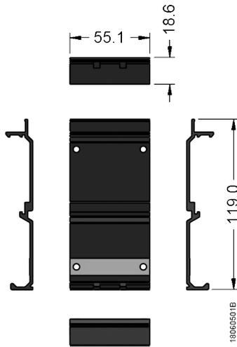
Figure 24: 2-Slot base for panel assembly
