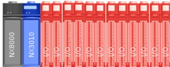
Figure 4: Single CPU with Nexto Jet Modules
